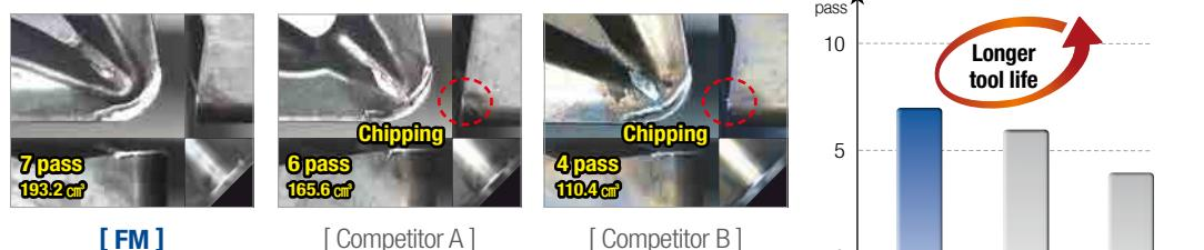
» Securing rigidity at the engagement boundary effectively prevents chipping and breakage at the boundary.
