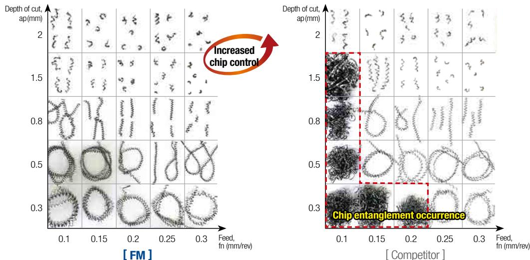
» Stable chip management and prevention of chip entanglement are achieved by the side V-shaped cutting edge and concave projection.
